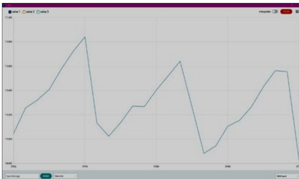
Fig 7: Output wave form of heart pulse using MAX30102
